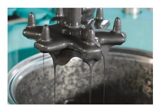
Not only do we need to protect the operators from the raw materials used in battery production, the raw materials itself, some of which are sensitive to moisture or oxygen, is almost always an issue and needs thorough attention when designing the system. AZO takes this into account with a special design in overlaying the handling process with inert gas or dry air.
